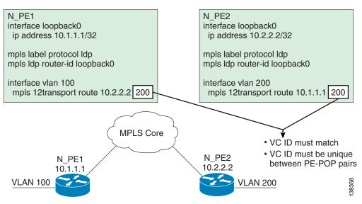
Note that the VC ID has to be the same on both ends of the EoMPLS tunnel. On each N-PE, there is mapping done between the VLANs to the EoMPLS tunnel. (See Figure E-5.)
